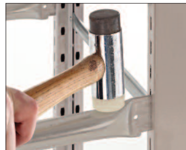
Tap down to locate beam into frame and insert locking pin. Beams easily repositioned using press and release locking pin system
